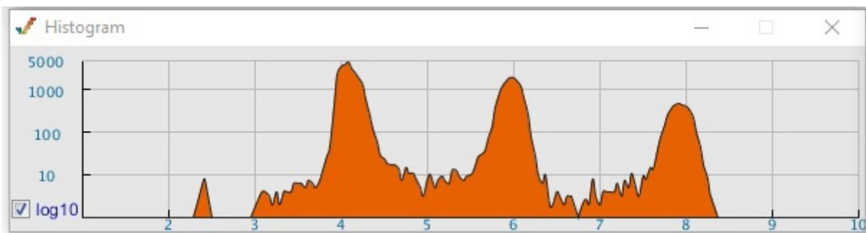
Now this is the damaged track from the second Fluxdetail example, here you can see that the transitions go all over the place, even with a small spike in the 2.5 $\mu$ s area. You can try formatting or erasing a disk like this and try again, if it still shows those signs, it will make a great coaster.
