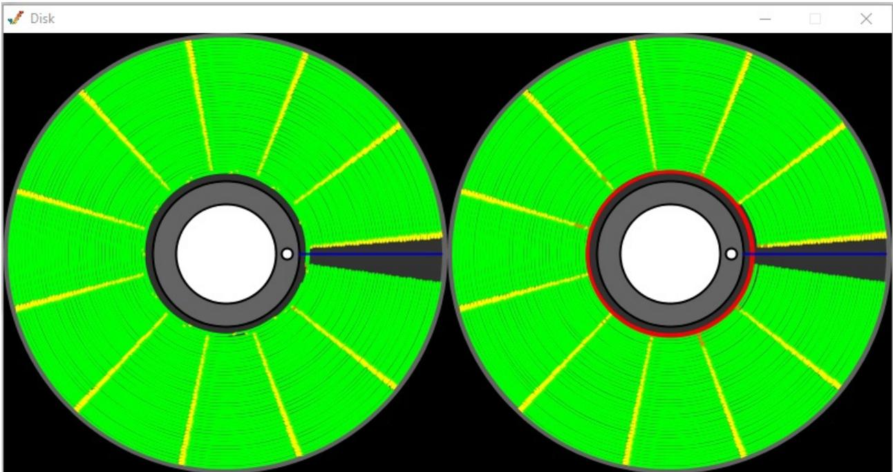
This shows a disk scan. Header areas are displayed yellow when the checksum is correct, orange when there is an error, data areas are displayed green when everything is fine, otherwise red when there is an error or no sectors found at all. The blue line marks the index hole.
