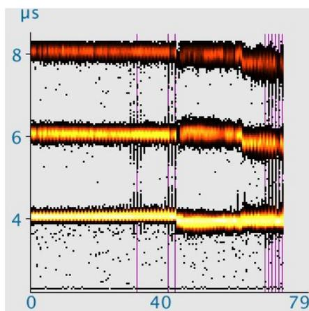
This shows the complete overview of a read, written or formatted disk when verify is on. The x axis are the tracks, the y-axis the transition time in microseconds. When retries were needed this is noted by a red vertical line. As you can see this disk is damaged in the higher tracks. The bands are getting very broad and there are a lot scattered transitions outside of the bands.
